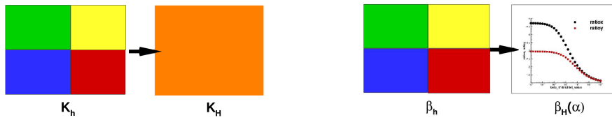
Fig. 1 Schematic difference between linear and nonlinear upscaling. Left: linear upscaling of \mathbf{K}_h delivers a constant upscaled value \mathbf{K}_H . Right: nonlinear upscaling of \beta_h delivers a map \beta_H(\alpha) where \alpha represents a local boundary condition value.
